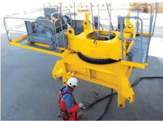
> After removal of the guardrail, the cab is rotated manually and locked in the working position.
