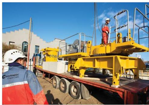
The winch is linked to the slewing unit in a single package
