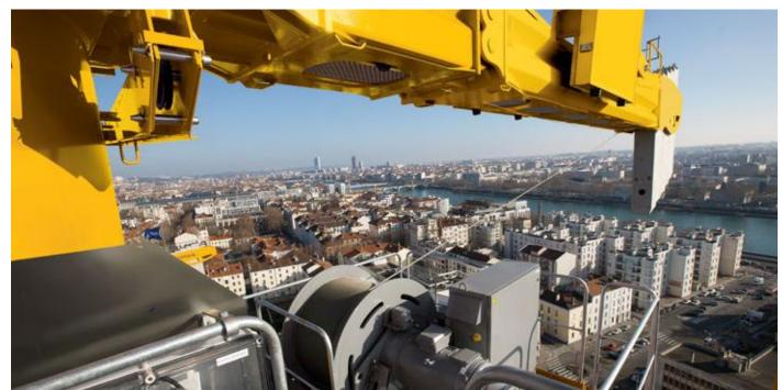
All mechanisms are accessible from the central area around the crane cabin.
